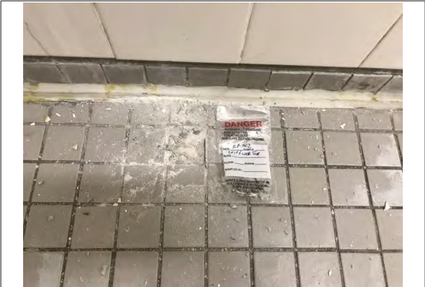
Picture No. 2: Sample 2 of grey ceramic floor tile for lead analysis – results indicate lead is present in the glaze at a concentration of 15.9mg/kg
