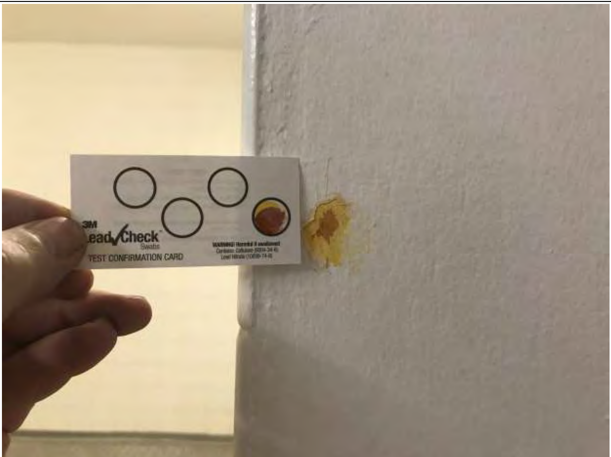
Picture No. 4: Swab analysis of painted wood – results indicate lead is present in the primer at a concentration greater than 600mg/kg
