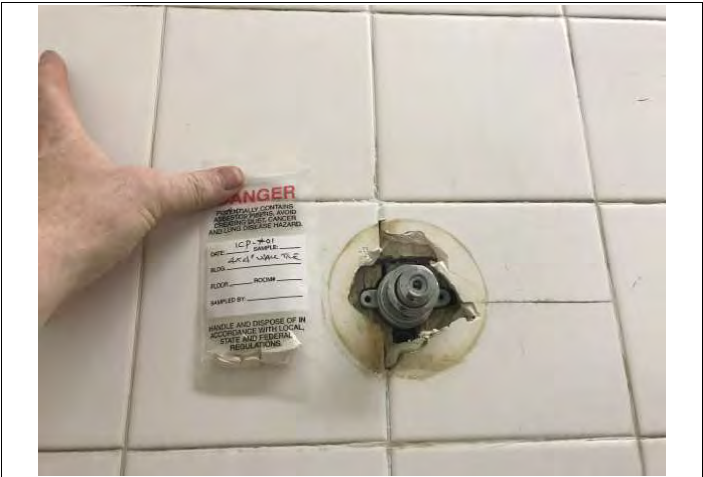
Picture No. 1: Sample 1 of white ceramic wall tile for lead analysis – results indicate lead is present in the glaze at a concentration of 292mg/kg
